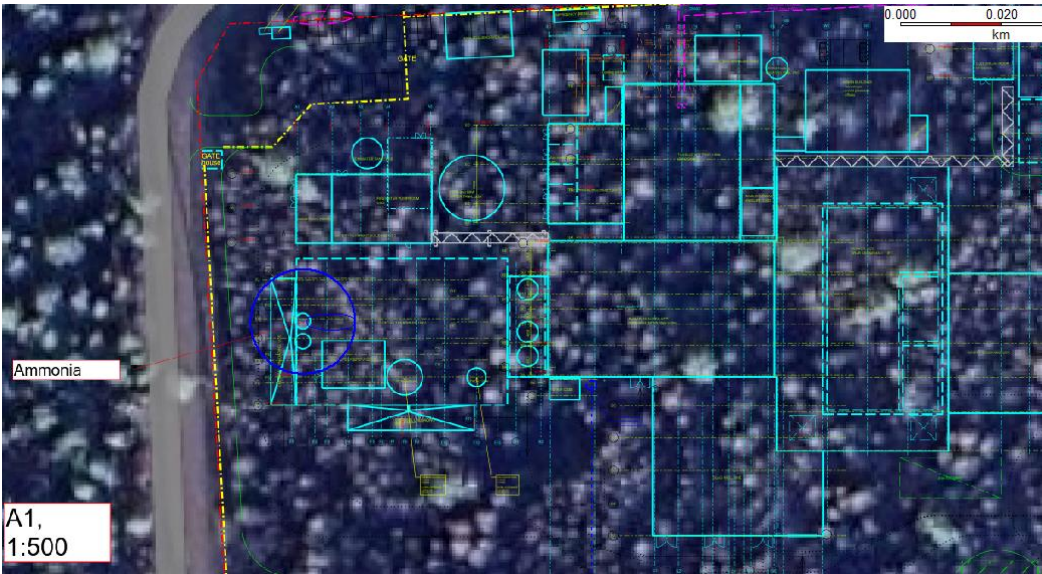
Figure 9: Distance (blue = 10 m) to 1 % lethality from ammonia release with 2 m/s wind. Smaller blue area is showing probability with one wind direction only (wind from west to east).
