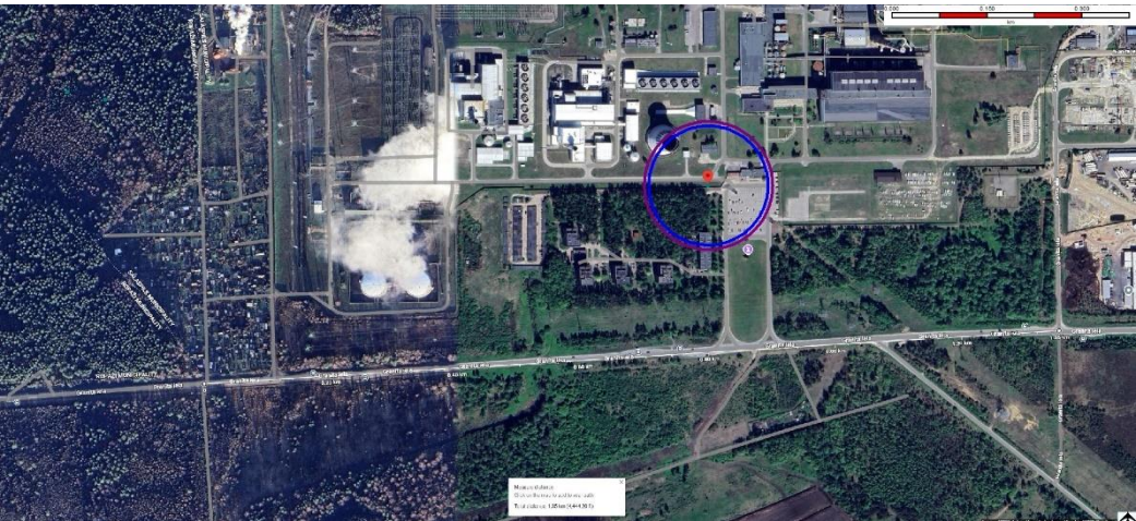
Figure 18: TEC-2 leakage related methane dispersion cloud as 100% lower flammability limit (44 000 ppm) seen above.
